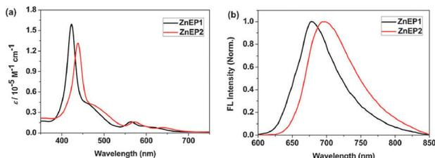
**Fig. 1** (a) Steady-state absorption and (b) fluorescence spectra of **ZnEP1** (black) and **ZnEP2** (red) recorded in CH<sub>2</sub>Cl<sub>2</sub>. Excitation was made in the Soret band.
