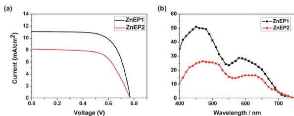
**Fig. 2** (a) Current–voltage characteristics and (b) action spectra at incident photon-to-current (IPCE) conversion efficiencies of DSSCs sensitized by **ZnEP1** (black) and **ZnEP2** (red). Conditions: [Co(bpy)<sub>3</sub>]<sup>2+</sup> based electrolyte in CH<sub>3</sub>CN and AM 1.5 under simulated solar light irradiation (100 mW cm<sup>-2</sup>).
