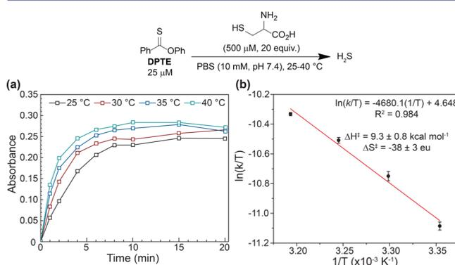
**Figure 6.** (a) Effect of temperature on rate of H<sub>2</sub>S release from DPTE (25 μM) in the presence of cysteine (500 μM, 20 equiv.). (b) Eyring analysis of H<sub>2</sub>S release from DPTE.
