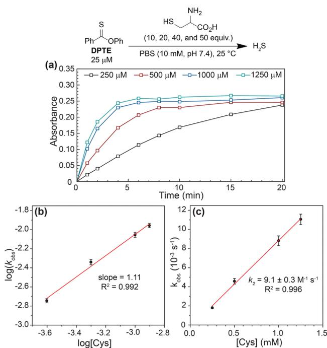
**Figure 5.** (a) H<sub>2</sub>S release by DPTE in the presence of increasing cysteine concentrations (250, 500, 1000, and 1250 μM). (b) Plot of log(*k*<sub>obs</sub>) vs log([Cys]) for DPTE. (c) Plot of *k*<sub>obs</sub> vs [Cys].
