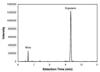
**Figure 3.** Ion chromatogram constructed from the SIM signal of m/z 237 (Mirex) between 6 and 9 min and the sum of SIM signals of m/z 337, 363, and 468 (TMS derivative of 5 ng/ $\mu$ L of ergosterol prepared in barley matrix) between 9 and 11 min.
