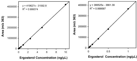
Figure 2. Standard calibration curves of ergosterol in the concentration ranges of  $0.025-10 \text{ ng}/\mu\text{L}$  (left) and  $0.025-1.0 \text{ ng}/\mu\text{L}$  (right) prepared in barley matrix.
