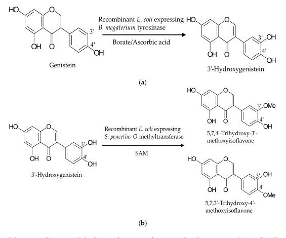
**Scheme 1.** Diagram of the biotransformation of genistein by the two recombinant *E. coli*. (a) Genistein was firstly biotransformed to 3'-hydroxygenistein by recombinant *E. coli* that expressed *B. megaterium* tyrosinase; (b) The produced 3'-hydroxygenistein was then biotransformed to 5,7,4'-trihydroxy-3'-methoxyisoflavone and 5,7,3'-trihydroxy-4'-methoxyisoflavone by recombinant *E. coli* that expressed *S. peucetius O*-methyltransferase.
