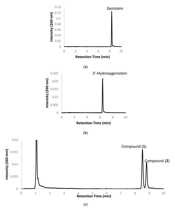
**Figure 1.** UPLC profiles of the biotransformation precursor genistein (**a**); the products of the first biotransformation reaction using the recombinant *E. coli* expressing tyrosinase (**b**); the products of the second biotransformation reaction using the recombinant *E. coli* expressing *O*-methyltransferase (**c**). The detailed protocols for biotransformation and UPLC are described in Materials and Methods.
