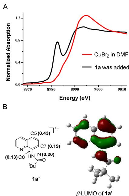
**Figure 1.** (A) XANES evidence for the single-electron transfer process between Cu(II) and **1a**. (B) Calculated Mulliken atomic spin densities (ASD) and lowest unoccupied molecular orbital ( $\beta$ -LUMO) of radical cation **1a'**.
