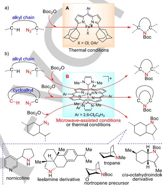
**Figure 2.** Examples of iron-catalyzed intramolecular C(sp<sup>3</sup>)-H amination of alkyl azides. a) Developed by Betley and co-workers using Fe-dipyrrinato catalysts **A**. b) Described in this work using Fe-NHC porphyrin catalyst **B**.
