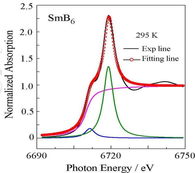
**Fig. 6** (Color online) The fitting results of normalized Sm  $L_3$  edge XANES spectra of SmB<sub>6</sub>
