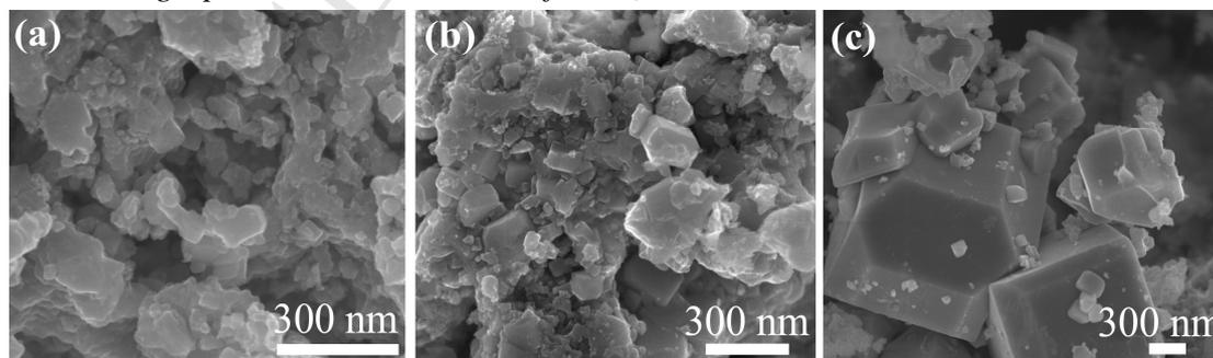
**Fig. 2** FESEM images of  $\text{SmB}_6$  prepared at different temperatures, using  $\text{Sm}_2\text{O}_3$  as raw materials, (a) 1000 °C for 4 h, (b) 1100 °C for 4 h, (c) 1100 °C for 20 h
