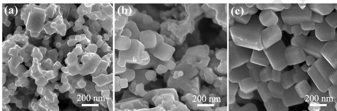
**Fig. 3** FESEM images of  $\text{SmB}_6$  prepared at different temperatures for 2 h, using  $\text{SmCl}_3$  as raw material, (a)  $1100\text{ }^\circ\text{C}$ , (b)  $1150\text{ }^\circ\text{C}$ , (c)  $1200\text{ }^\circ\text{C}$
