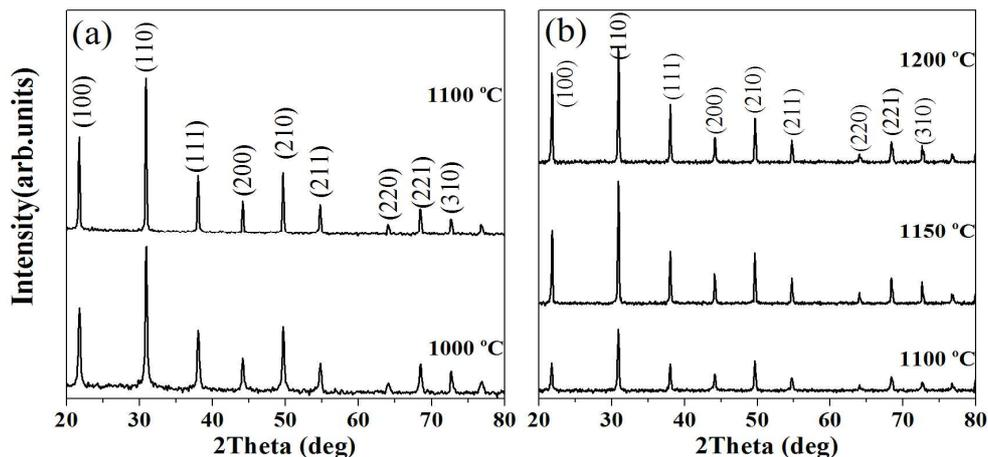
**Fig. 1** XRD patterns of  $\text{SmB}_6$  powder synthesized at different temperatures, (a) prepared  $\text{Sm}_2\text{O}_3$  as raw material, (b) prepared  $\text{SmCl}_3$  as raw material
