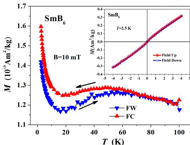
**Fig. 7** (Color online) Temperature dependence of the magnetization of  $\text{SmB}_6$  nanoparticles measured under ZFC and FC conditions in an applied field of 10 mT. Inset shows the full  $M(H)$  loop of  $\text{SmB}_6$  measured at 2.5 K.
