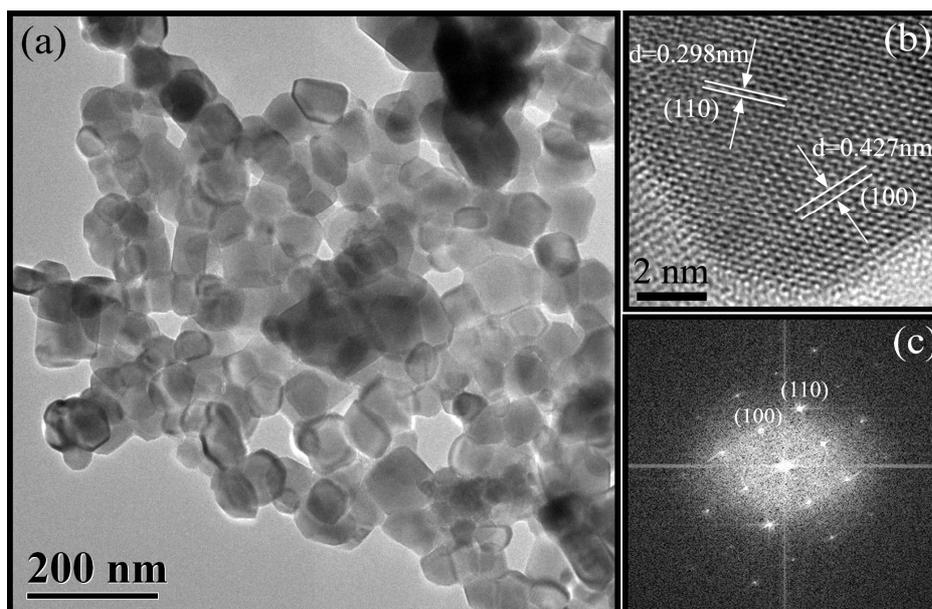
**Fig. 4** (a) TEM analyses of  $\text{SmB}_6$  nanocrystalline, (b) the HRTEM image (top right), (c) the indexing FFT patterns (down left).
