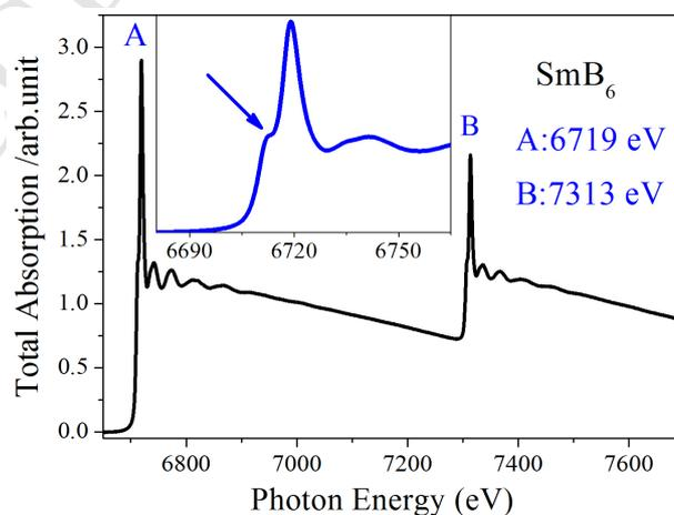
**Fig. 5** (Color online) The total X-ray absorption spectra of  $\text{SmB}_6$  nanoparticles against photon
