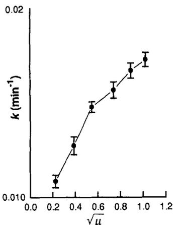
**Figure 8**—Dependence of log  $k$  of OQZ (214  $\mu$ M) on  $\sqrt{\mu}$  in  $\text{CH}_3\text{CN}$ :0.0625 N NaOH (1:4; v/v) containing (data points from left to right) 0, 0.1, 0.25, 0.5, 0.75, and 1 M NaCl, respectively, at 25 °C.
