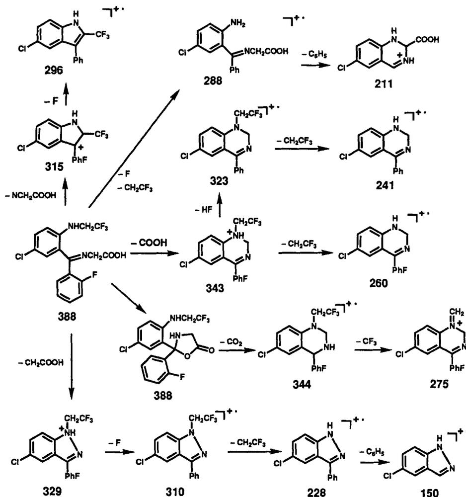
**Scheme 1**—Some fragmentation pathways proposed to account for some of the major mass fragments observed in the electron impact mass spectrum of OQZ-HP (PhF and Ph are abbreviations for 2'-fluorophenyl and phenyl groups, respectively).
