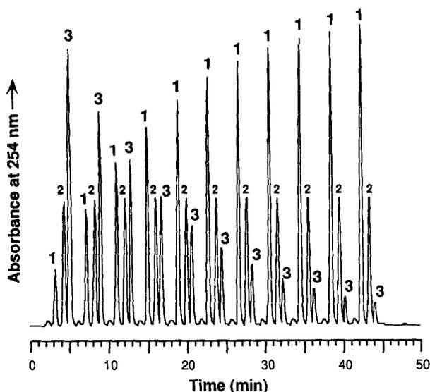
**Figure 2**—An example of the time course in the monitoring of OQZ hydrolysis by reversed-phase HPLC. Hydrolysis of OQZ was conducted in  $\text{CH}_3\text{CN}:0.2 \text{ N NaOH}$  (1:1, v/v) at  $25^\circ\text{C}$ . Samples ( $10 \mu\text{L}$  each injection) were repetitively injected every 3.92 min. The hydrolysis  $t_{1/2}$  of this reaction was 10.4 min.
