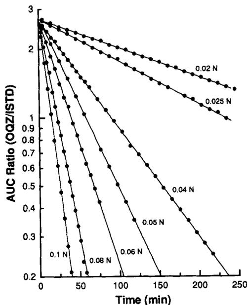
**Figure 6**—Dependence of hydrolysis rate of OQZ (214  $\mu\text{M}$ ) on [NaOH] in  $\text{CH}_3\text{CN}:\text{H}_2\text{O}$  (1:1; v/v) at  $25^\circ \text{C}$ . Disappearance of OQZ was expressed by the normalized AUC ratio of [OQZ]:[ISTD]. The final concentration of NaOH for each determination is indicated.
