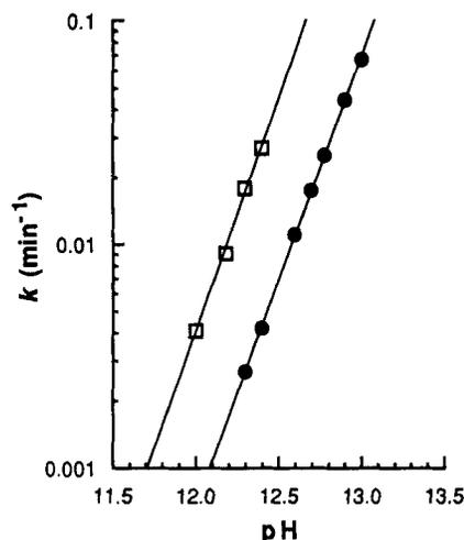
**Figure 7**—Dependence of  $\log k$  or OQZ (214  $\mu\text{M}$ ) on [NaOH] in  $\text{CH}_3\text{CN}:\text{H}_2\text{O}$  [(□) 3:1 or (●) 1:1; v/v] at  $25^\circ \text{C}$ . The concentration of NaOH is expressed by pH, which is equal to  $14 + \log [\text{NaOH}]$ . The slopes of the two lines are (□) 2.08 and (●) 2.01.
