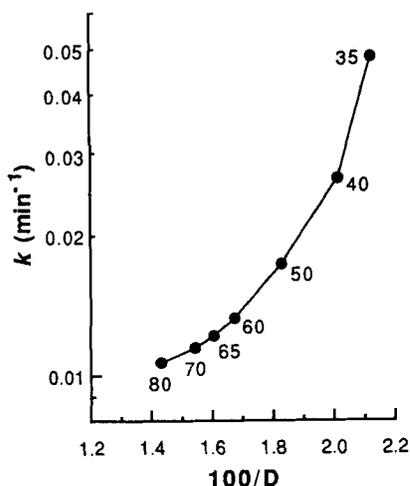
**Figure 9**—Dependence of log  $k$  of OQZ (214  $\mu$ M) on  $100/D$  in various volume ratios of  $\text{CH}_3\text{CN}$ : $\text{H}_2\text{O}$  containing 0.05 N final concentration of NaOH at 25 °C ( $D$  is the weighted dielectric constant of the solvent; see text for explanation). The volume percentage of water contained in the solvent mixture is indicated next to each data point.
