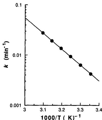
**Figure 10**—Arrhenius plot for temperature dependence of log  $k$  in the hydrolysis of OQZ. The hydrolysis reaction was conducted in  $\text{CH}_3\text{CN}$ :0.05 N NaOH (1:1, v/v). Slope, -3.15;  $E_{\text{act}} = 14.4$  kcal/mol;  $\Delta H^\ddagger = 13.8$  kcal/mol (at 25 °C);  $\Delta S^\ddagger = -31.2$  cal/K/mol (at 25 °C);  $\Delta G^\ddagger = 23.1$  cal/mol (at 25 °C).
