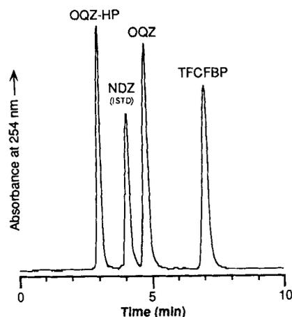
**Figure 1**—Reversed-phase HPLC separation of OQZ-HP, NDZ, OQZ, and TFCFBP. Chromatographic conditions are described in the *Experimental Section*.
