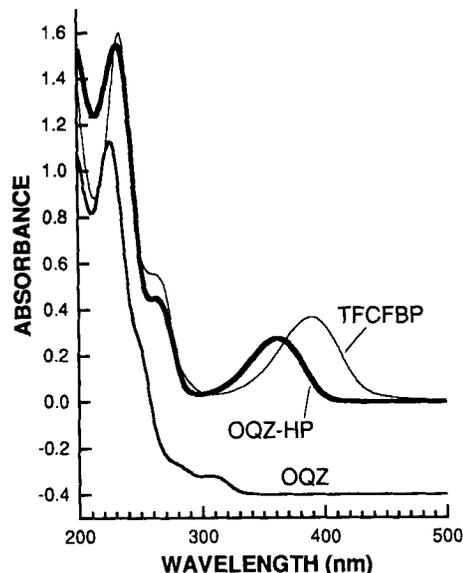
**Figure 3**—UV-vis absorption spectra of OQZ [ $43 \mu\text{M}$ ; characteristic  $\lambda_{\text{max}}$  at 226, 249 (sh), and 309 nm], OQZ-HP (characteristic  $\lambda_{\text{max}}$  at 233, 263, and 362 nm), and TFCFBP (characteristic  $\lambda_{\text{max}}$  at 234, 262, and 389 nm) in  $\text{CH}_3\text{CN}$ . The absorbance of OQZ is offset by 0.4 absorbance unit to avoid excessive overlapping of curves.
