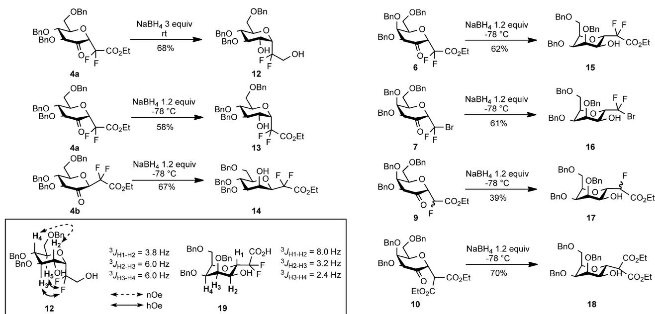
Scheme 4. Reduction of 2-ketohexopyranosides **4** and **6–10** with sodium borohydride.
