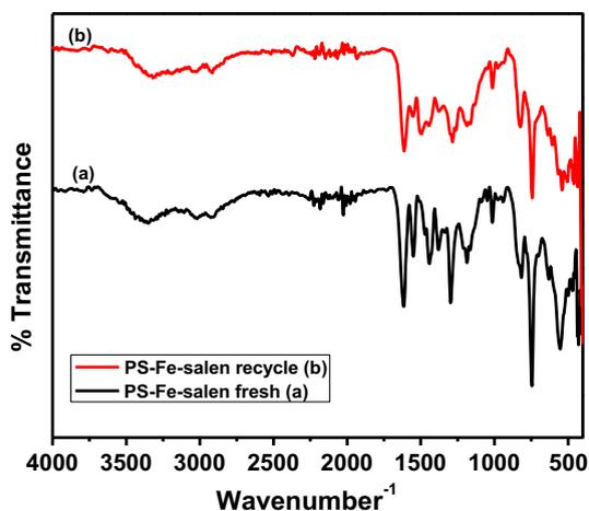
Fig. 4 FT-IR spectra of PS–Fe–salen before and after reaction
