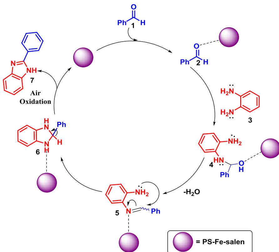
**Fig. 3** Plausible mechanism for synthesis of 2-phenylbenzimidazole catalyzed by PS–Fe–salen
