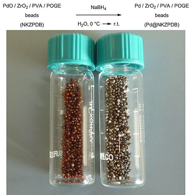
Fig. 1. Sketch of the synthesis of the hybrid catalytic materials with abbreviations adopted (top). Images of NKZPDB-1 beads (bottom), before (left) and after (right) palladium reduction.
