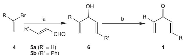
**Scheme 2** Synthesis of divinylketones **1** from  $\alpha$ -bromostyrenes **4**. Reagents and conditions: (a) 1. *n*-BuLi, THF, 1.5 h,  $-78^\circ\text{C}$ ; 2. aldehyde **5**, 1.5 h,  $-78^\circ\text{C}$ ; (b) excess  $\text{MnO}_2$ ,  $\text{CH}_2\text{Cl}_2$ , 60 min,  $23^\circ\text{C}$ .
