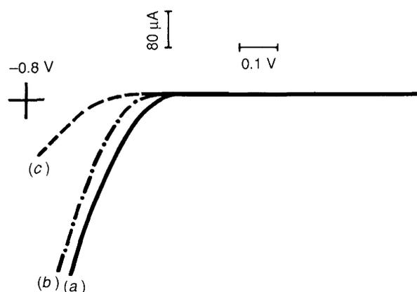
**Fig. 1** Reduction of oxygen on  $\text{TiO}_2$  and modified  $\text{TiO}_2$  electrodes in  $0.2 \text{ mol dm}^{-3} \text{ NaClO}_4$ . Sweep rate:  $20 \text{ mV s}^{-1}$ . (a)  $\text{TiO}_2$ , (b)  $\text{TiO}_2$ -sil- $\text{Fe}^{\text{III}}(\text{tpps})$  and (c)  $\text{TiO}_2$ -sil.
