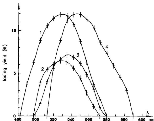
Fig. 3. Lasing yield and tuning range of: 1,  $\text{BP(OH)}_2$ ; 2,  $\text{MeBP(OH)}_2$ ; 3,  $\text{Me}_2\text{BP(OH)}_2$  in cyclohexane; 4, coumarin 153 in ethyl alcohol.
