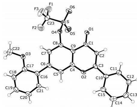
Figure 1. Ortep plot of **7e**. Ellipses are drawn at the 50% probability level.<sup>[21]</sup>
