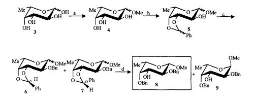
Conditions: a. MeOH, TsOH, reflux, 24 h; quant. b. PhCH(OMe)<sub>2</sub>, TsOH, DMF, 45 °C, 5 h; 57% c. i. NaH, DMF, rt, 0.5 h; ii. BnBr, DMF, 10 h; 91% d. DIBAL, CH<sub>2</sub>Cl<sub>2</sub>, 0 °C, 3 h; 92%
