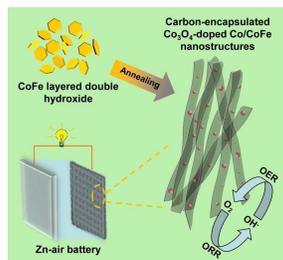
Carbon-encapsulated Co<sub>3</sub>O<sub>4</sub>-doped Co/CoFe bifunctional catalyst prepared by annealing LDH acts as a highly efficient air cathode in rechargeable Zn-air battery.
