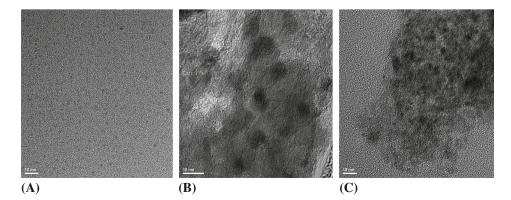
Figure 2. TEM images of (A): Pd colloid; (B): IM-Pd/Al<sub>2</sub>O<sub>3</sub>; (C) CD-Pd/Al<sub>2</sub>O<sub>3</sub> catalyst.
