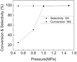
**Figure 4.** Effect of pressure on hydrogenation of MA over CD-Pd/Al<sub>2</sub>O<sub>3</sub> catalyst. Reaction conditions: T = 353 K, P = 1.0 MPa, catalyst: 0.1 g, MA = 7.35 g.
