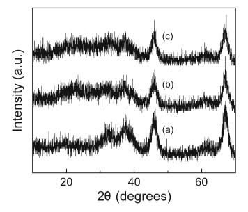
Figure 1. XRD patterns of (a)  $Al_2O_3$  support; (b) IM-Pd/Al\_2O\_3; (c) CD-Pd/Al\_2O\_3 catalyst.
