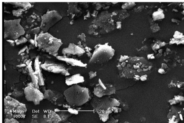
Fig. 1 The SEM image for the prepared pretreatment cellulose particles.
