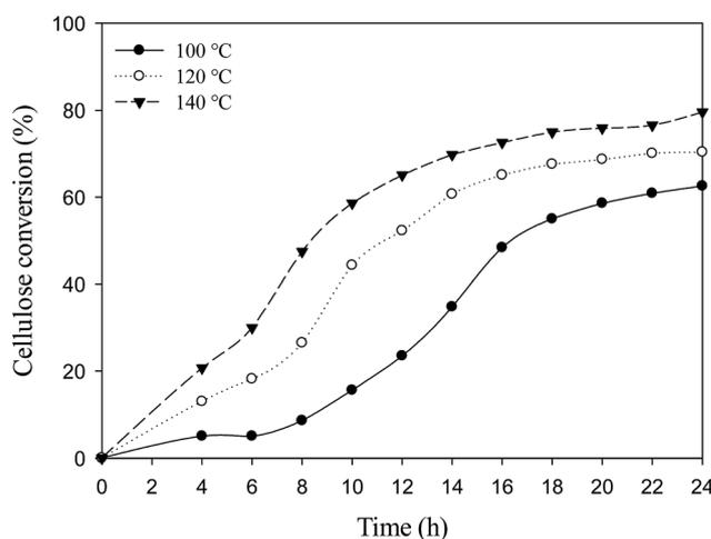
Fig. 4 Effects of hydrolysis temperature on the cellulose conversion (pretreated cellulose, 0.05 g; catalyst, 0.1 g; water, 4 mL).
