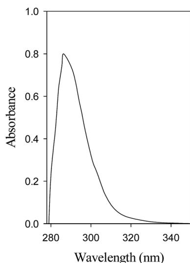
Fig. 8 UV spectrum of the hydrolysis products of cellulose.
