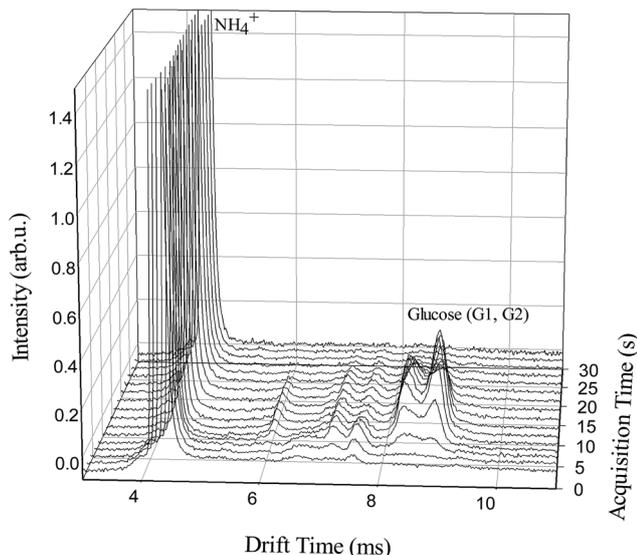
Fig. 7 The section of the watershed 3D plots of the ion mobility spectra of glucose.
