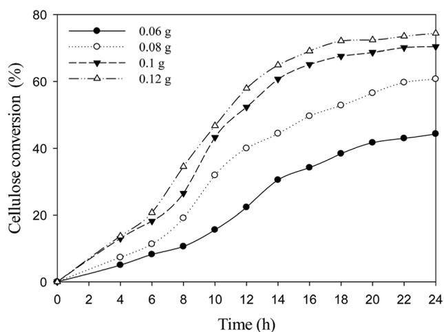
Fig. 3 Effects of catalyst amount on the cellulose conversion (pretreated cellulose, 0.05 g; water, 4 mL; reaction temperature, 120 °C).
