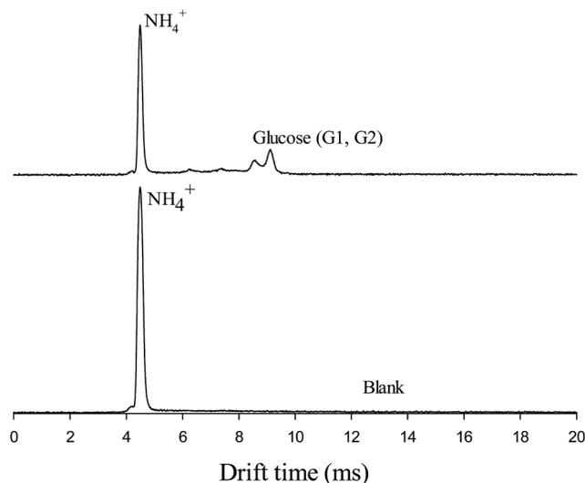
Fig. 5 The ion mobility spectra of the glucose and blank.
