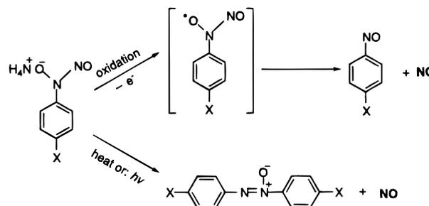
Cupferron, an analogue of diazeniumdiolate, is commonly used in industry as a metal chelator<sup>19</sup> and a polymerization inhibitor.<sup>20</sup> It is also a donor that can release NO upon enzymatic,<sup>21</sup> electrochemical,<sup>22,23</sup> as well as chemical oxidation.<sup>24</sup> Hwu et al. also discovered that cupferron can thermally and photochemically decompose to azoxy compounds and release NO (Scheme 1).<sup>25</sup>
