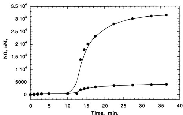
**Figure 4.** Chemical release of NO from *N*-(*N'*-acetylphenylalanylmethylenyloxy)-*N*-phenyldiimide *N*-oxide (**14**). The compound was dissolved at 6.0 mM in a mixture of CH<sub>3</sub>CN and phosphate buffer (10 mM with 1.0 mM EDTA) (1/1 (v/v)). Top line, pH, 11.0; Bottom line, pH 8.0.
