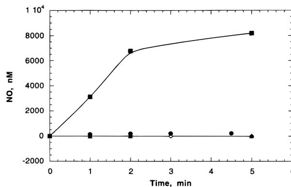
**Figure 1.** Stability of cupferron and its *O*-alkyl derivatives at 25 °C: (■) cupferron, (◇) *N*-(*o*-nitrobenzyl)oxy-*N*-phenyldiimide *N*-oxide (**12**), (▲) *N*-methoxy-*N*-phenyldiimide *N*-oxide (**1**), and (●) *N*-(*N*'-acetylphenylalanylmethylenoxy)-*N*-phenyldiimide *N*-oxide (**14**). The NO donors were dissolved at 6.0 mM in a mixture of CH<sub>3</sub>CN and phosphate buffer (10 mM, pH 7.0, with 1.0 mM EDTA) (4/1 (v/v)). The solutions were deoxygenated with argon.
