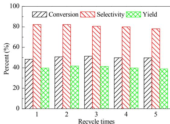
**Fig. 7.** Recyclability of the Ru-Zn-3 catalyst for the selective hydrogenation of benzene to cyclohexene. Reaction conditions: Ru-Zn-3 catalyst 0.12 g, ZrO<sub>2</sub> 0.6 g, ZnSO<sub>4</sub>·7H<sub>2</sub>O 8.4 g, C<sub>6</sub>H<sub>6</sub> 35 mL, H<sub>2</sub>O 70 mL, 150 °C, 5 MPa of H<sub>2</sub> pressure, stirring rate 1200 r/min, 45 min.
