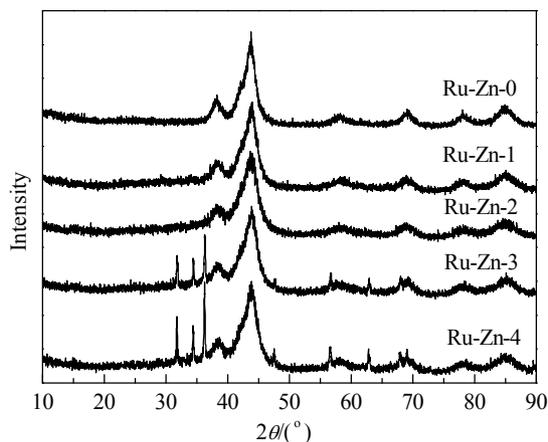
Fig. 1. XRD patterns of the Ru-Zn catalysts with different Zn contents.
