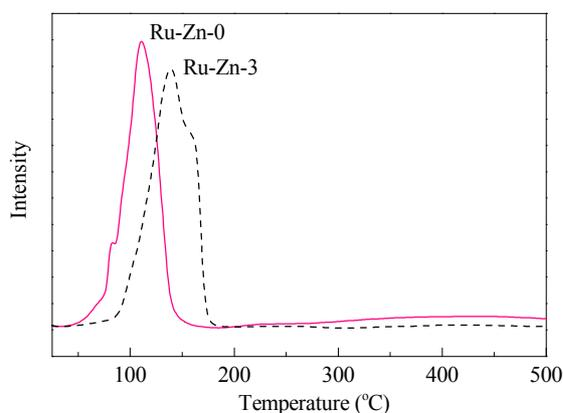
Fig. 2.  $\text{H}_2$ -TPR profiles of catalysts Ru-Zn-0 and Ru-Zn-3 before reduction.
