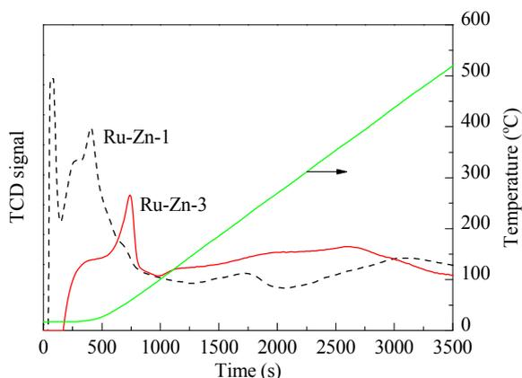
Fig. 4. H<sub>2</sub>-TPR profiles of catalysts Ru-Zn-1 and Ru-Zn-3 after reduction.
