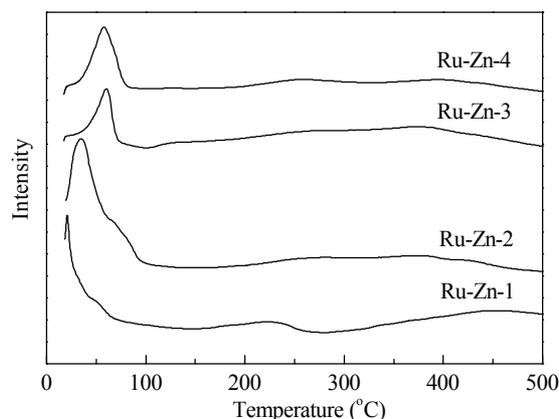
Fig. 3.  $\text{H}_2$ -TPR profiles of Ru-Zn catalysts with different Zn contents after reduction.
