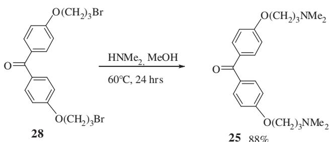
Scheme 1. Synthesis of 4,4'-bis-dimethylaminopropoxy-benzophenone **25**.
