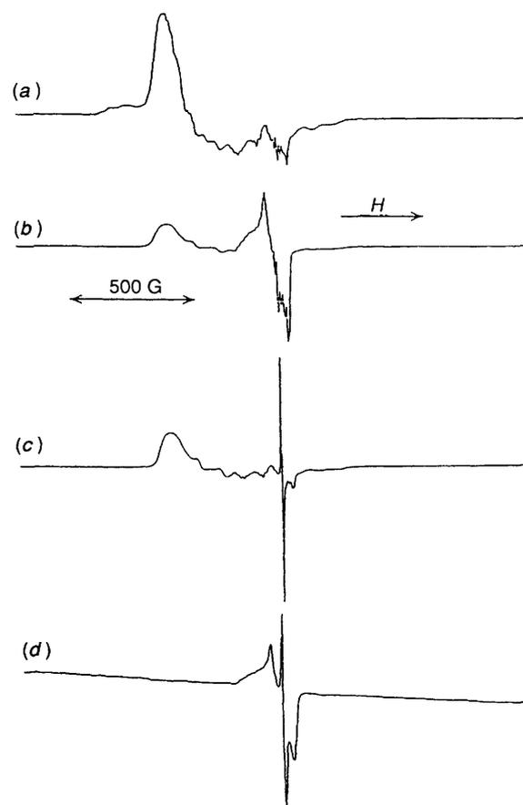
**Fig. 3** The ESR spectra of the reaction mixture after 1 h at  $-196\text{ }^\circ\text{C}$ . The reaction was catalysed by  $[\text{Co}(\text{babp})]$  at (a) 20, (b) 40 and (c)  $60\text{ }^\circ\text{C}$  and by  $[\text{Co}(\text{salen})]$  at  $40\text{ }^\circ\text{C}$  (d)
