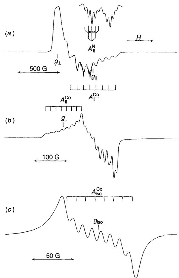
**Fig. 1** The ESR spectra of  $[\text{Co}(\text{mbabp})]$  in toluene-pyridine: (a) under anaerobic conditions at  $-196\text{ }^\circ\text{C}$  ( $g_{\perp}$  2.31,  $g_{\parallel}$  2.032,  $A_{\parallel}^{\text{N}}$  77.4 G, and  $A_{\parallel}^{\text{Co}}$  14.0 G for  $[\text{Co}(\text{mbabp})(\text{py})_2]$ ), (b) under oxygenated conditions at  $-196\text{ }^\circ\text{C}$  (ESR parameters in Table 2), and (c) under aerobic conditions at  $-71\text{ }^\circ\text{C}$
