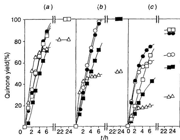
**Fig. 2** Oxidation reactions catalysed by cobalt(II) complexes. Substrate:  $0.5\text{ mol dm}^{-3}$ . Catalyst:  $2.5 \times 10^{-3}\text{ mol dm}^{-3}$ . Temperature: (a) 20, (b) 40 and (c)  $60\text{ }^\circ\text{C}$ . Complexes: (○)  $[\text{Co}(\text{babp})]$ , (●)  $[\text{Co}(\text{mbabp})]$ , (□)  $[\text{Co}(\text{bbabp})]$ , (■)  $[\text{Co}(\text{cbabp})]$  and (△)  $[\text{Co}(\text{salen})]$
