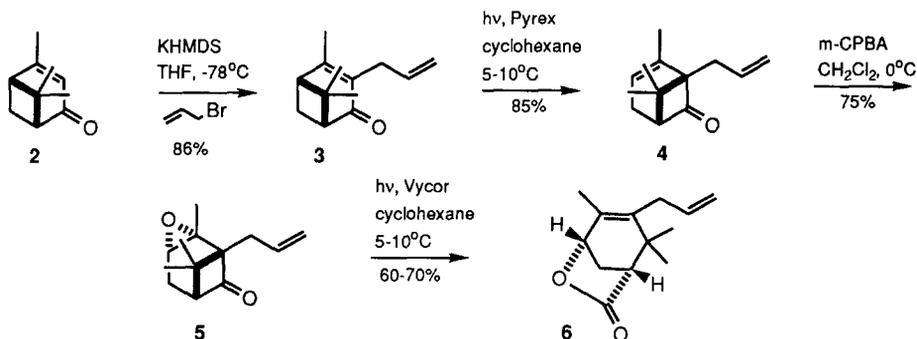
The requisite C-13 oxygen functionality of taxol was introduced via regioselective and stereoselective epoxidation of **4** from the least hindered face (away from the geminal dimethyl group) of the more highly substituted alkene to give **5**. Based on the pioneering work of Agosta and Murray,<sup>10</sup> the  $\beta,\gamma$ -ketoepoxide **5** underwent a second photochemically mediated rearrangement to yield the  $\gamma$ -lactone, **6**.
