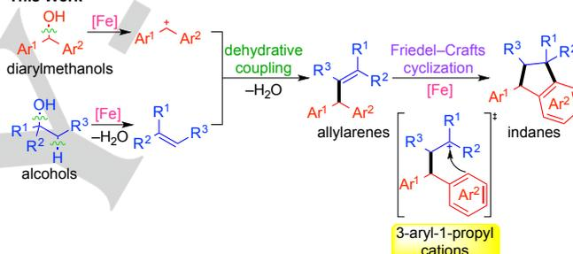
**Scheme 1.** Iron-catalyzed direct synthesis of indanes from two different alcohols.
