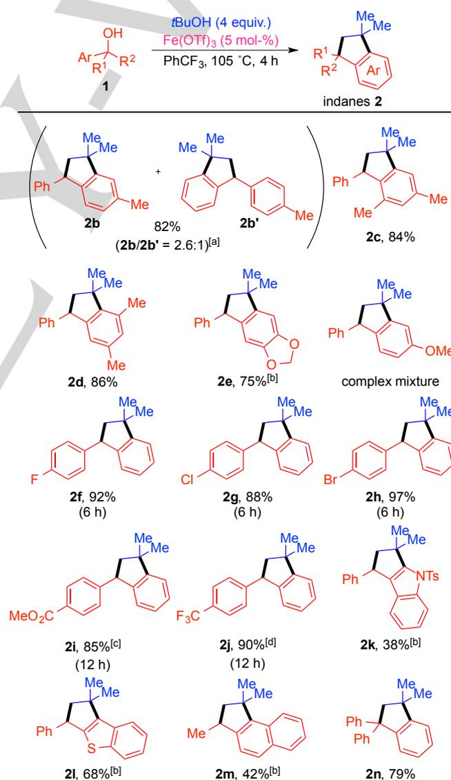
**Scheme 2.** Iron-catalyzed regioselective synthesis of indanes. Reaction conditions: **1** (0.25 mmol), *t*BuOH (1.0 mmol), and Fe(OTf)<sub>3</sub> (5 mol-%) in
