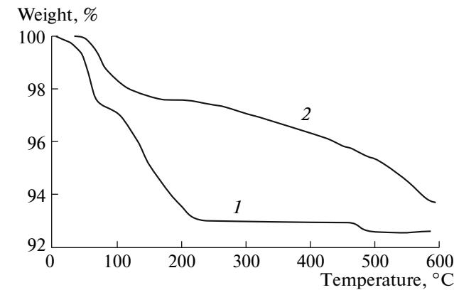
**Fig. 1.** TGA of TPA (1) and  $\text{TPA}_3/\text{SiO}_2$  (2).
