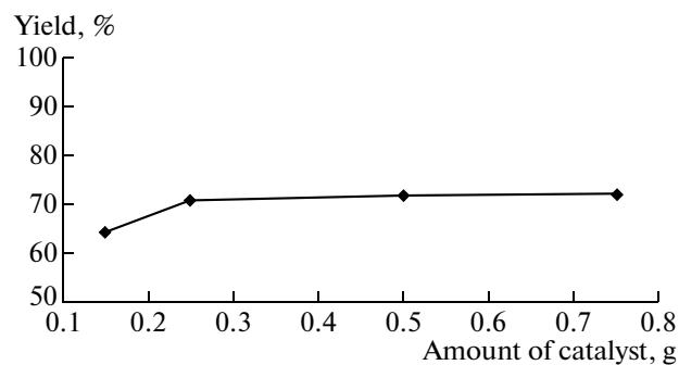
**Fig. 5.** The yield of butyl acetate with TPA<sub>3</sub>/SiO<sub>2</sub> catalyst (molar ratio of alcohol to acid is 1 : 4.4).
