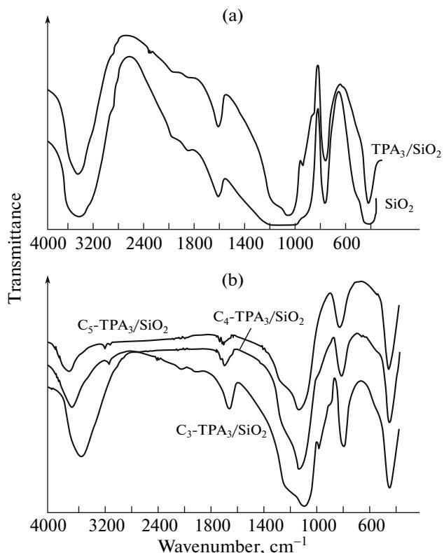
Fig. 3. (a) FT-IR spectra of  $\text{SiO}_2$  and  $\text{TPA}_3/\text{SiO}_2$ ; (b) FT-IR spectra of  $\text{C}_3\text{-TPA}_3/\text{SiO}_2$ ,  $\text{C}_4\text{-TPA}_3/\text{SiO}_2$ , and  $\text{C}_5\text{-TPA}_3/\text{SiO}_2$ .
