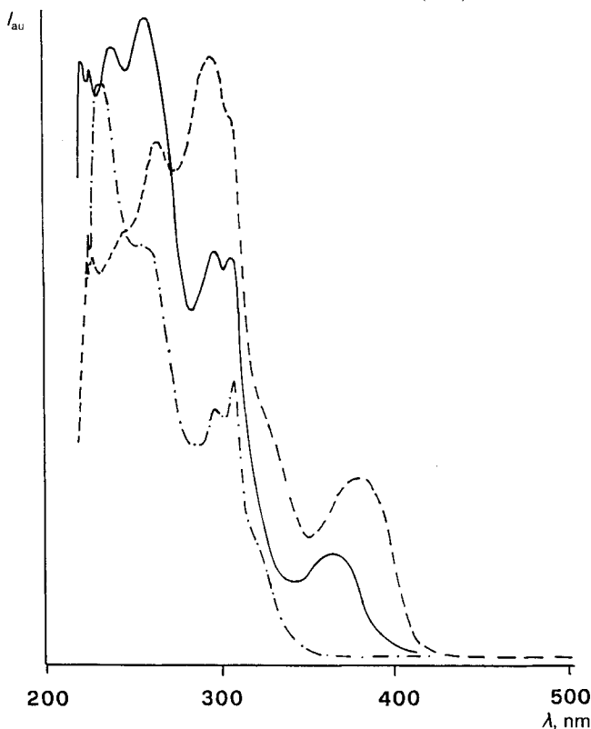
Fig. 2. UV/VIS Spectra in \text{CH}_2\text{Cl}_2 of [\text{Rh}(\text{2-thpy})_2(\text{bpy})]^+ (---), [\text{Rh}(\text{ppy})_2(\text{bpy})]^+ (—), and [\text{Rh}(\text{ppz})_2(\text{bpy})]^+ (-·-·-)
