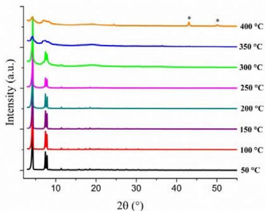
**Figure 6:** VTXPDP plots of **K[CFA-4]** in the range of 50-400°C. \*peaks belong to Cu phase (PDF no. 4-836).
