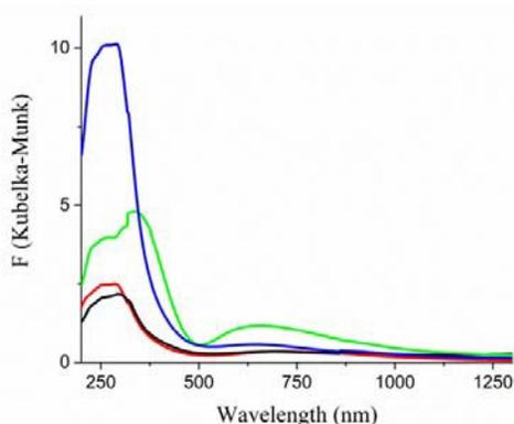
**Figure 13:** UV-vis spectra of **M[CFA-4]** at room temperature. Red line: **K[CFA-4]** freshly prepared; black line: **Cu(I)[CFA-4]** freshly prepared; green line: **Cu[CFA-4]** oxidised; blue line: **Cu(I)[CFA-4]** reduced.
