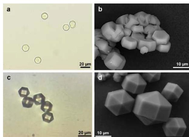
**Figure 1** **Cu(I)[CFA-4]**: (a) optical micrograph after synthesis in DMF as solvent; (b) SEM image after synthesis in DMF as solvent; (c) optical micrograph after synthesis with solvent methanol and 2,6-lutidine; (d) SEM image after synthesis with solvent methanol and 2,6-lutidine.
