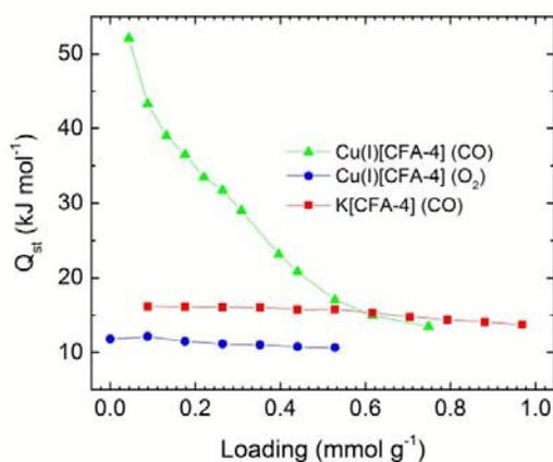
**Figure 8:** Isosteric heats of CO (green) and  $\text{O}_2$  (blue) adsorption in **Cu(I)[CFA-4]** and CO adsorption in **K[CFA-4]** (red).
