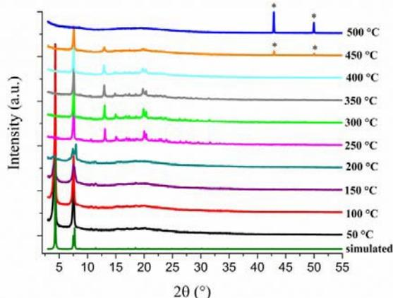
**Figure 5:** VTXPDP plots of **Cu(I)[CFA-4]** in the range of 50-500°C. The dark green XRPD pattern is simulated based on single crystal X-ray data. \*peaks belong to Cu phase (PDF no. 4-836).
