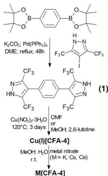
**Scheme 1** Syntheses of 1,4-bis(3,5-bis(trifluoromethyl)-*lH*-pyrazole-4-yl)benzene **1**, **Cu(I)[CFA-4]** and **M[CFA-4]** (DME = 1,2-dimethoxyethane).
