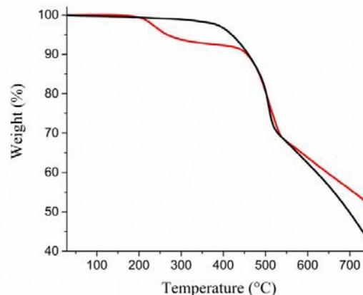
**Figure 4:** Temperature dependent weight loss of **Cu(I)[CFA-4]** (red line) and **K[CFA-4]** (black line) under flowing nitrogen gas.
