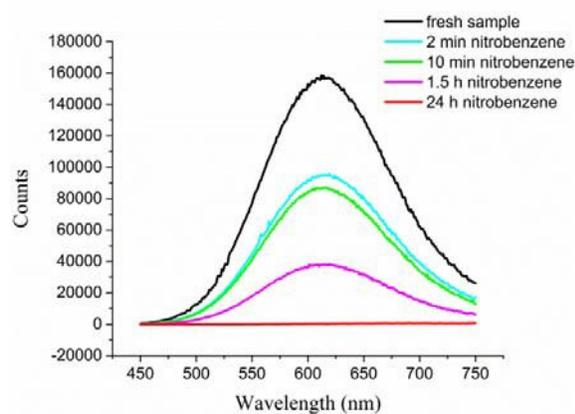
**Figure 12:** Solid-state photoluminescence spectra of **Cu(I)[CFA-4]** exposed to a nitrobenzene vapour at room temperature for various time periods (excitation wavelength 320 nm).
