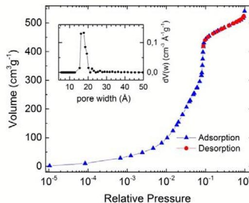
**Figure 7:** Argon adsorption (blue) and desorption (red) isotherms of **K[CFA-4]** at 87 K. Inset: pore size distribution calculated from these isotherms.
