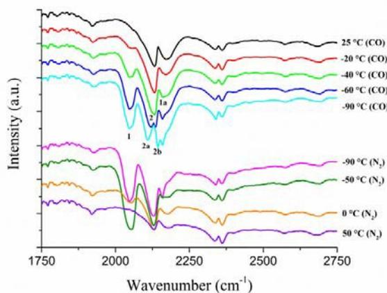
**Figure 9:** In situ DRIFT spectra of **Cu(I)[CFA-4]** upon cooling from room temperature to  $-90 \text{ }^\circ\text{C}$  under CO atmosphere and subsequent heating from  $-90 \text{ }^\circ\text{C}$  to  $50 \text{ }^\circ\text{C}$  under  $\text{N}_2$  atmosphere.
