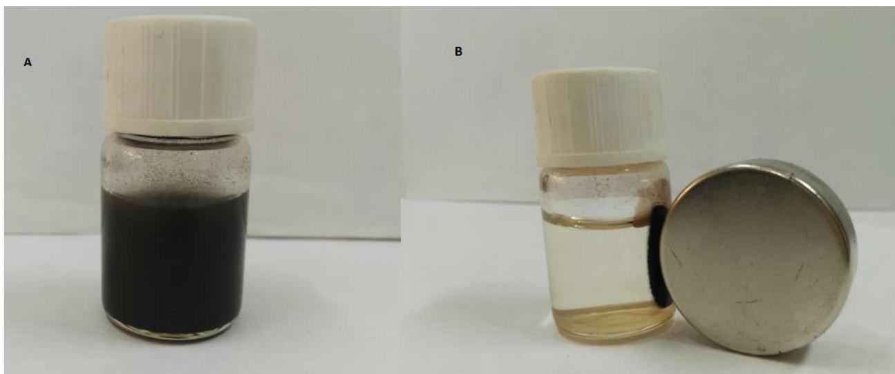
**Fig. 9. Photograph of the aqueous solution A, with dispersed Pd-Schiff-Base@Fe<sub>3</sub>O<sub>4</sub>MNPs and B after 5 second applied magnetic field**
