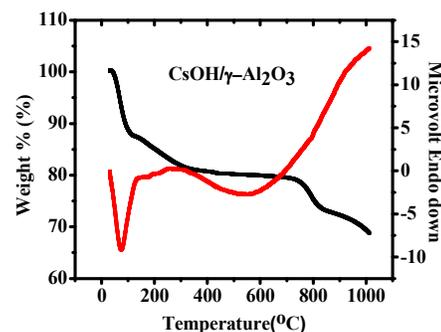
**Fig.3** TG-DTA analysis of CsOH/  $\gamma\text{-Al}_2\text{O}_3$  catalyst
