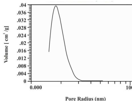
**Fig. 6** BJH pore size distribution curve of CsOH/  $\gamma$ -Al<sub>2</sub>O<sub>3</sub> catalyst
