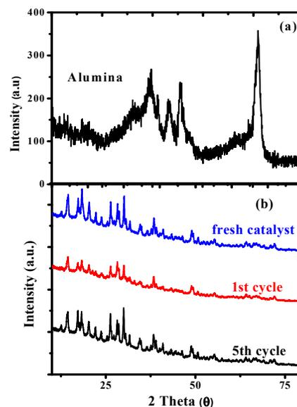
**Fig.2** XRD patterns of (a)  $\gamma\text{-Al}_2\text{O}_3$  and (b) CsOH/  $\gamma\text{-Al}_2\text{O}_3$  calcined at  $400^\circ\text{C}$  i. fresh catalyst ii. 1<sup>st</sup> cycle iii. 5<sup>th</sup> cycle of reuse.
