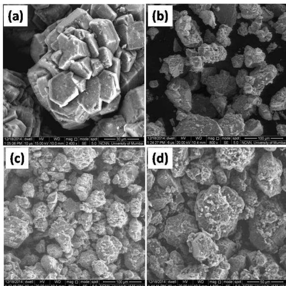
**Fig. 4** SEM images of (a)  $\gamma$ -Al<sub>2</sub>O<sub>3</sub> (b) CsOH/  $\gamma$ -Al<sub>2</sub>O<sub>3</sub> before reaction (c) CsOH/  $\gamma$ -Al<sub>2</sub>O<sub>3</sub> after 1<sup>st</sup> recycle reaction (d) CsOH/  $\gamma$ -Al<sub>2</sub>O<sub>3</sub> after 5<sup>th</sup> recycle reaction.
