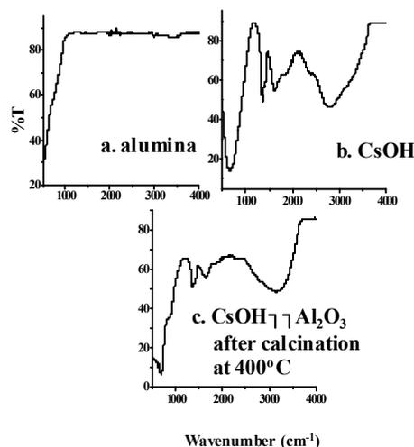
**Fig.1** FT-IR spectra of (a)  $\gamma\text{-Al}_2\text{O}_3$ , (b) CsOH, (c) CsOH/  $\gamma\text{-Al}_2\text{O}_3$  catalyst after calcination at  $400^\circ\text{C}$ .
