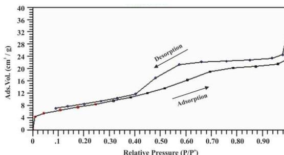
**Fig. 5** N<sub>2</sub> adsorption-desorption isotherm of CsOH/  $\gamma$ -Al<sub>2</sub>O<sub>3</sub> catalyst.
