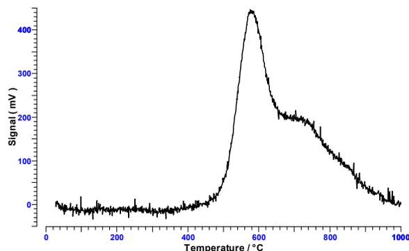
**Fig. 7** CO<sub>2</sub>-TPD analysis of the catalyst CsOH/ $\gamma$ -Al<sub>2</sub>O<sub>3</sub>
