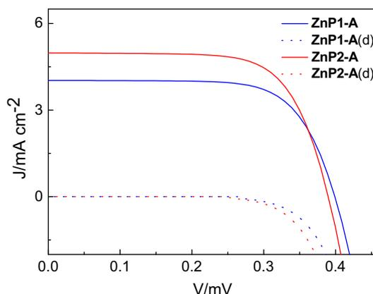
Figure 5. *J*–*V* characteristics of **ZnP<sub>x</sub>-A**-sensitized SC measured under irradiance of 100 mW cm<sup>-2</sup> AM 1.5G sunlight (**ZnP<sub>x</sub>-A**) and in the dark (**ZnP<sub>x</sub>-A(d)**).
