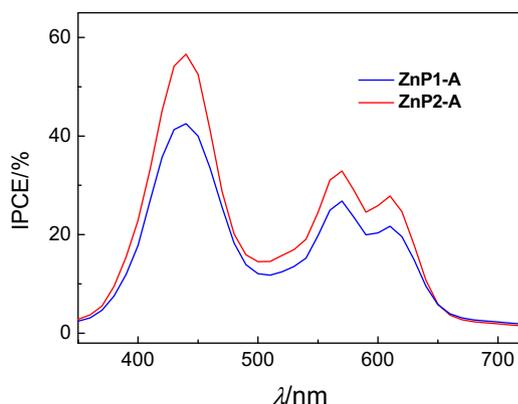
Figure 4. Photocurrent action spectra of **ZnP<sub>x</sub>-A**-sensitized solar cells.
