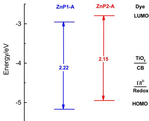
Figure 3. Orbital energy-levels of these assemblies, TiO<sub>2</sub>, and electrolyte I<sup>3-</sup>/I<sup>-</sup>.
