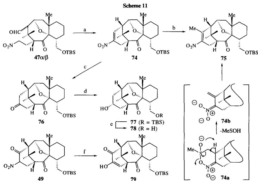
Conditions:- a) Tetramethylguanidine/CH<sub>2</sub>Cl<sub>2</sub>/24h, followed by MeSO<sub>2</sub>Cl/DBU, **74** (64%). b) LiCH<sub>2</sub>S(O)Me/THF/0°C, **75** (45%). c) NaBH<sub>4</sub>/MeOH/0°C, followed by H<sub>2</sub>O<sub>2</sub>/K<sub>2</sub>CO<sub>3</sub>, **76** (60%). d) DIBAL-H/CH<sub>2</sub>Cl<sub>2</sub>/-78°C, **77** (84%). e) HF.py/THF, **78** (91%). f) MeONa/MeOH/O<sub>3</sub>, followed by Me<sub>2</sub>S, **79** (51%).
