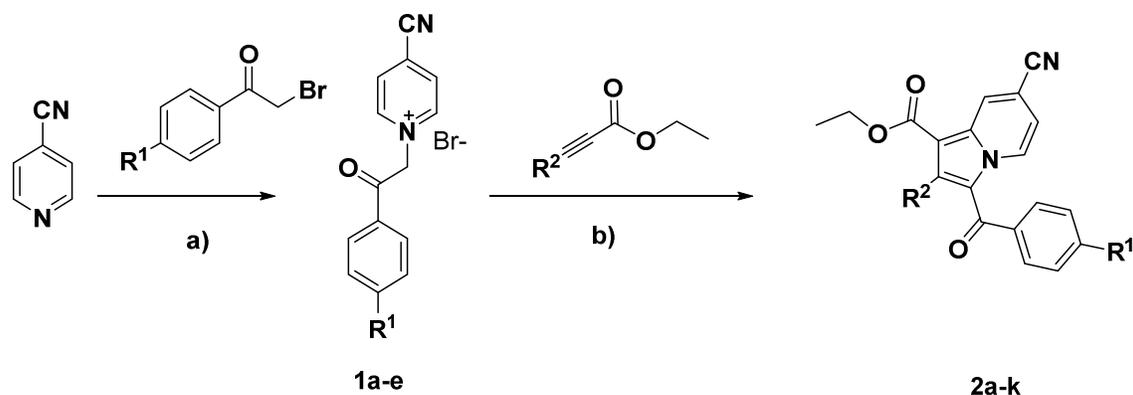
**Scheme 1** Synthetic scheme for the construction of novel indolizine scaffolds (**2a-k**): (a) acetone, r.t., 5h; (b) DMF,  $\text{K}_2\text{CO}_3$ , 30 min.
