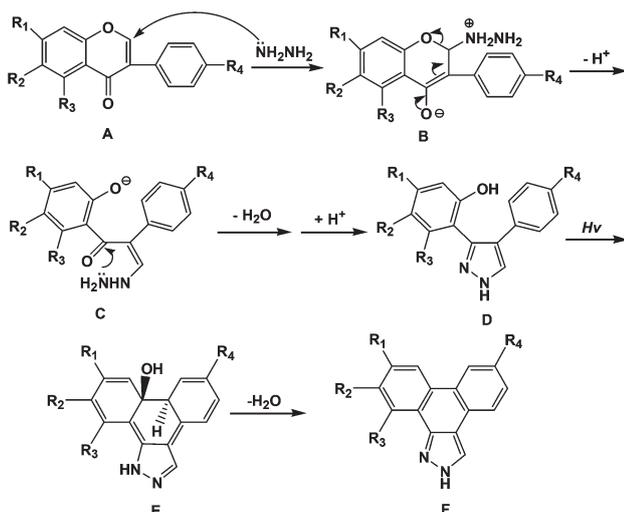
**Scheme 3** Proposed mechanism for two dehydration processes.
