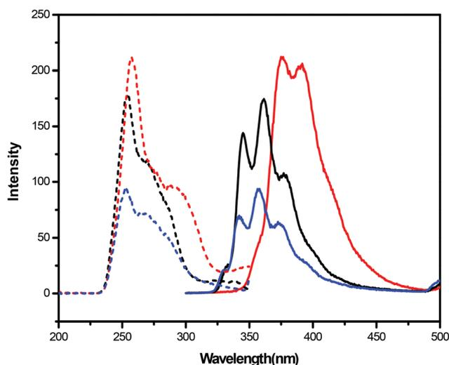
Fig. 1 Excitation spectra (EX, dash lines) and emission spectra (EM, solid lines) of compounds **1i** (red), **1a** (black) and **1p** (blue) in chloroform ( $1 \times 10^{-6}$  mol  $L^{-1}$ ).
