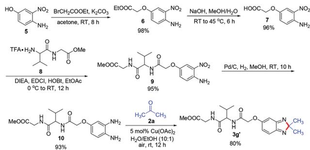
**Scheme 2** Synthesis of 2,2-methyl 2*H*-benzo[*d*]imidazole derivative (**3g'**) containing dipeptide in aqueous medium (DIEA = *N,N*-diisopropylethylamine, EDCI = 1-ethyl-3-(3-dimethylaminopropyl)carbodiimide hydrochloride, HOBT = *N*-hydroxybenzotriazole).
