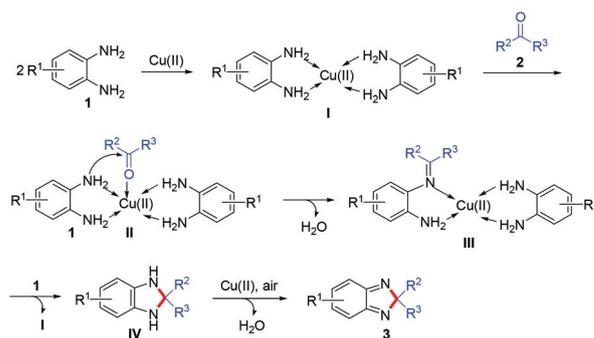
**Scheme 5** Possible mechanism for copper-catalyzed conjugations of *o*-aromatic diamines with ketones.
