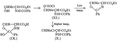
By carrying out the cyclisation slowly at low temperature, a very good yield of the oxazoline was obtained, and the formation of the chloro-compound was entirely suppressed. The mixture
