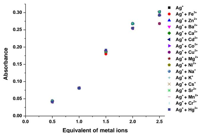
**Figure 5.** UV-vis absorbance of receptor **1** (10  $\mu$ M) at 426 nm in the presence of various metal ions in water (10 mM HEPES, pH 7.5).
