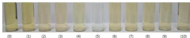
**Figure 8.** Color changes in the complex **1**-Ag (10  $\mu$ M) upon addition of anions (5 equiv). [(0): **1**-Ag complex, (1):  $\text{F}^-$ , (2):  $\text{Br}^-$ , (3):  $\text{Cl}^-$ , (4):  $\text{ClO}_4^-$ , (5):  $\text{I}^-$ , (6):  $\text{CN}^-$ , (7):  $\text{NO}_3^-$ , (8):  $\text{OAc}^-$ , (9):  $\text{HSO}_4^-$ , and (10):  $\text{H}_2\text{PO}_4^-$ ].
