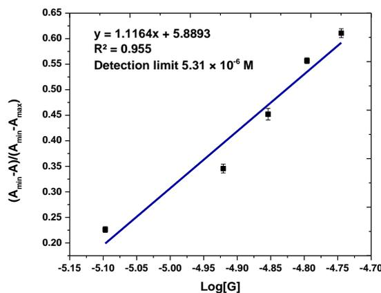
**Figure 10.** Detection limit of the complex **1**-Ag for estimation of  $\Gamma$ .
