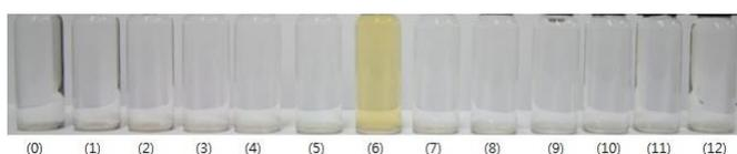
**Figure 3.** Photographic images of receptor **1** (10  $\mu\text{M}$ ) in water (10 mM HEPES, pH 7.5) in the presence of metal ions (5 equiv) (From 0 to 12: receptor **1**,  $\text{Cu}^{2+}$ ,  $\text{Fe}^{3+}$ ,  $\text{Zn}^{2+}$ ,  $\text{Ni}^{2+}$ ,  $\text{Mg}^{2+}$ ,  $\text{Ag}^+$ ,  $\text{Co}^{2+}$ ,  $\text{Cd}^{2+}$ ,  $\text{Ca}^{2+}$ ,  $\text{Ba}^{2+}$ ,  $\text{Na}^+$ , and  $\text{K}^+$ ).
