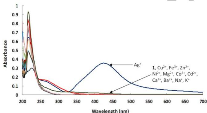
**Figure 1.** UV-vis absorbance of receptor **1** (10  $\mu\text{M}$ ) upon addition of particular metal (5 equiv) in water (10 mM HEPES, pH 7.5).
