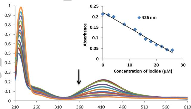
**Figure 9.** Absorbance changes in the complex **1**-Ag (10  $\mu$ M) upon addition of  $\Gamma$  (0-2.6 equiv) in water (10 mM HEPES, pH 7.5).
