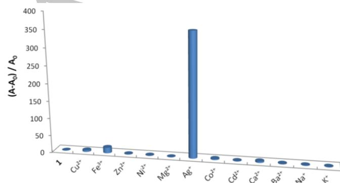
**Figure 2.** UV-vis absorbance of receptor **1** (10  $\mu\text{M}$ ) upon addition of particular metal (5 equiv) in water (10 mM HEPES, pH 7.5) at 426 nm.
