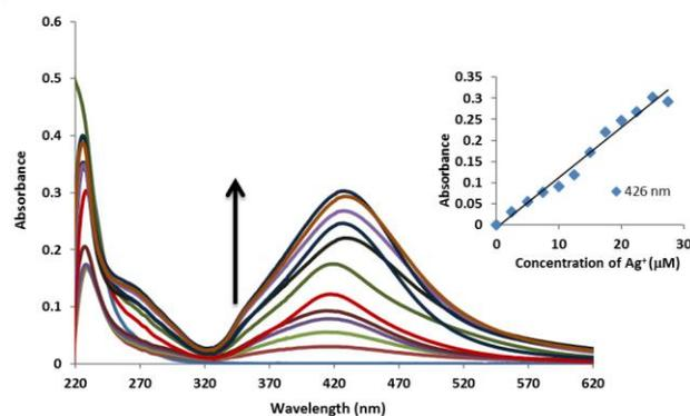
**Figure 4.** Absorbance changes in receptor **1** (10  $\mu\text{M}$ ) upon addition of  $\text{Ag}^+$  ions (0-2.7 equiv) in water (10 mM HEPES, pH 7.5).
