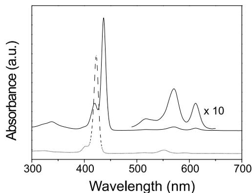
Fig. 1. Electronic absorption spectrum of Ga(TPP)H (solid line) and Ga(TPP)Cl (dashed line) in toluene.
