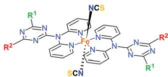
**Scheme 2** Representation of the *trans*-[Fe<sup>II</sup>L<sub>2</sub>(NCS)<sub>2</sub>] complexes whose structural and SCO properties are described in Table 4. **R**<sup>1</sup> and **R**<sup>2</sup> symbolize different substituents on the triazine ring (see Table 4).
