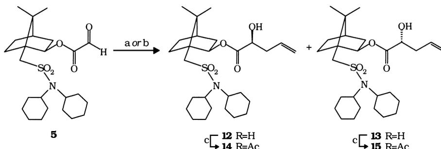
Scheme 5. Reagents and reaction conditions: (a) allylmagnesium chloride,  $-78^{\circ}\text{C}$ , THF; (b) allyltrimethylsilane, Lewis acid,  $\text{CH}_2\text{Cl}_2$ , the other conditions: see Table 2; (c)  $\text{Ac}_2\text{O}$ , py, rt, 3 h
