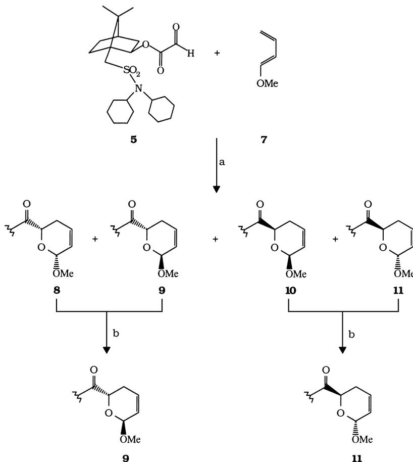
Scheme 3. Reagents and reaction conditions: (a) 20°C, CH<sub>2</sub>Cl<sub>2</sub>, the amounts of catalyst and the pressure are indicated in Table 1; (b) PPTS, MeOH, rt, overnight
