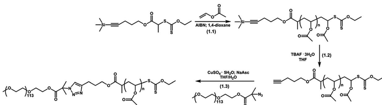
Fig. 15 Schematic representation of the RAFT polymerization of VAc (1.1), PVAc deprotection (1.2) and synthesis of PEG-*b*-PVAc block copolymers by CuAAC reaction (1.3).
