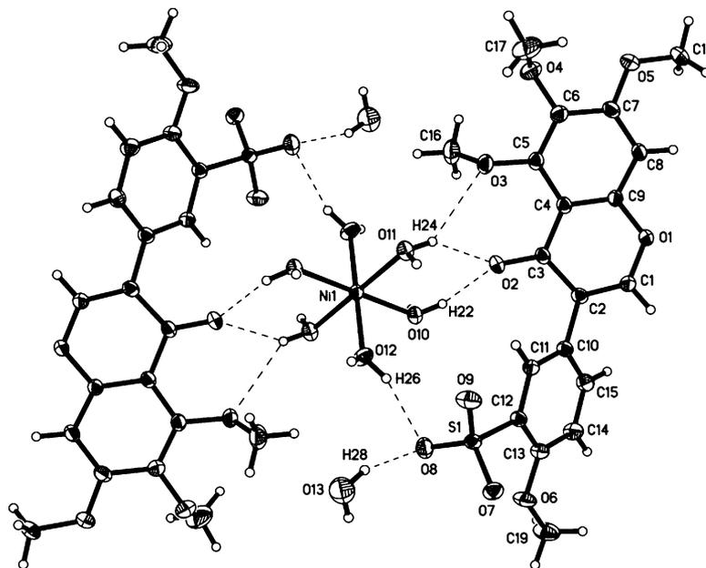
**Fig. 1.** Molecular structure of the title compound showing 30% probability displacement ellipsoids. Thin dashed lines indicate O–H···O hydrogen bonds.
