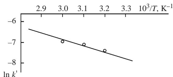
Fig. 5. Plot of  $\ln k'$  vs. reciprocal temperature for the reduction of  $VO[L^3]$ .
