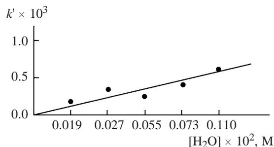
**Fig. 4.** Pseudo-first-order rate constant *k'* of the reduction of VO[L<sup>3</sup>] at 22°C as a function of [H<sub>2</sub>O]. [NaBH<sub>4</sub>] 0.002 M.
