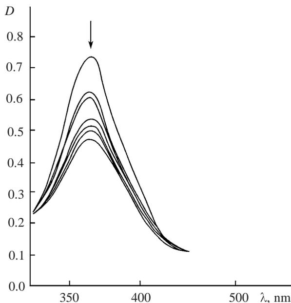
**Fig. 1.** Variation with time of the absorption intensity in the electronic spectra of  $\text{VO}[\text{L}^3]$ .  $T$  35°C,  $[\text{NaBH}_4]$  0.002 M,  $[\text{H}_2\text{O}]$  0.073 M. The spectra were recorded at 2-min intervals. The arrow denotes the direction of spectrum evolution. ( $D$ ) Optical density.
