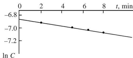
**Fig. 2.** Logarithm of the substrate concentration as a function of time for the reduction of  $\text{VO}[\text{L}^3]$ . Initial concentrations, M:  $\text{VO}[\text{L}^3]$   $1 \times 10^{-4}$ ,  $[\text{NaBH}_4]$  0.002, and  $[\text{H}_2\text{O}]$  0.073.
