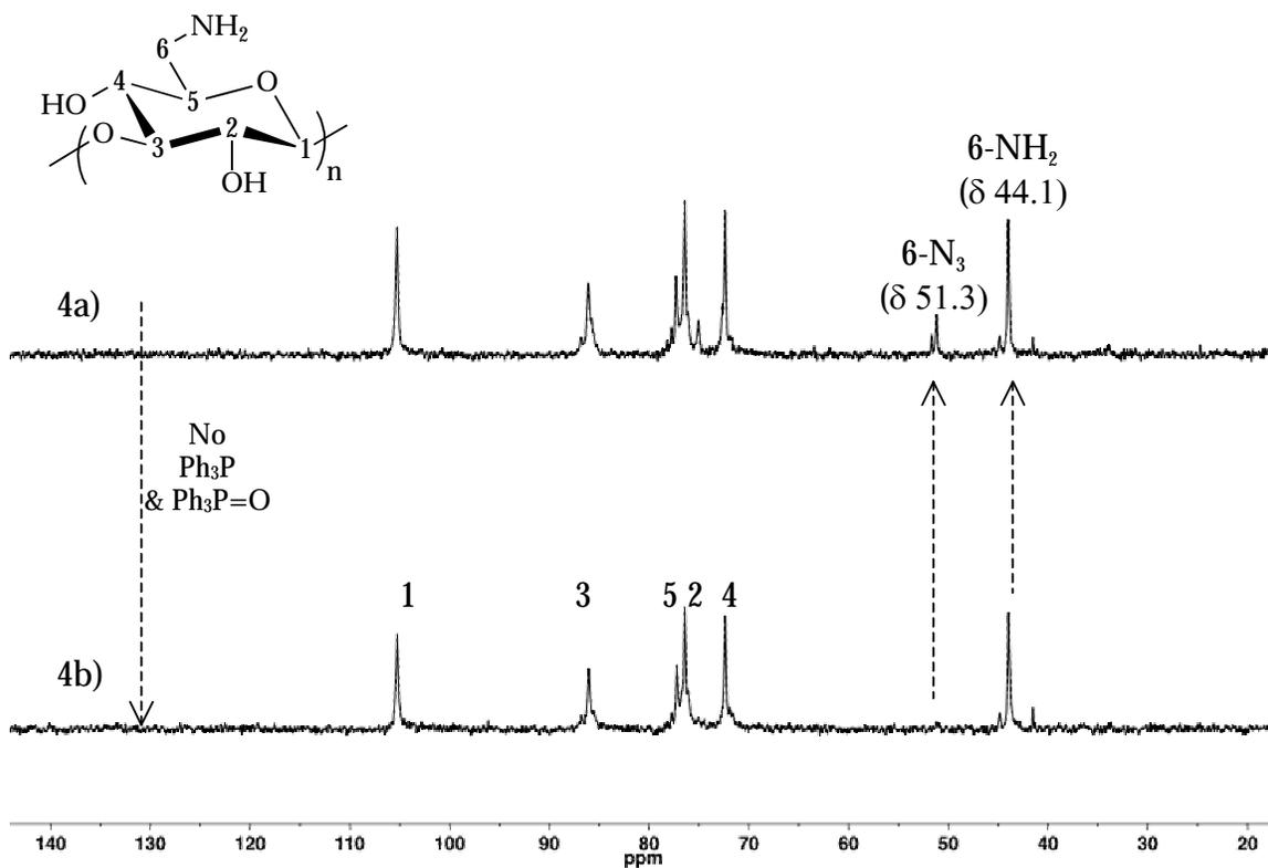
474 Figure 4.  $^{13}\text{C}$  NMR spectra of 6-amino-6-deoxycurdlan: 4a) 60°C, 24 h and 4b) 100°C, 24 h.
