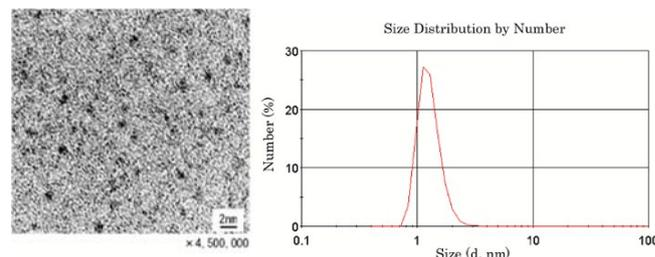
**Fig. 1** Left: Transmission electron microscopy image of DMF-stabilized Ir nanoclusters (NCs). Bar length: 2 nm. Right: Dynamic light scattering spectrum of Ir NCs.
