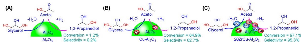
Figure 4. Proposed reaction pathway for glycerol hydrogenolysis in \text{Al}_2\text{O}_3 (A), \text{Cu-Al}_2\text{O}_3 (B) and 20\text{ZrCu-Al}_2\text{O}_3 (C).
