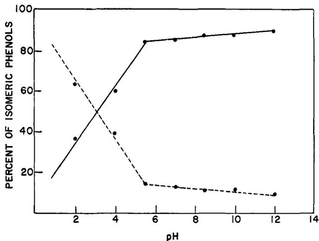
FIGURE 1: Isomerization of 1,4-dimethylbenzene 1,2-oxide (**12**) to 2,4-dimethylphenol (**19**, ●—●) and 2,5-dimethylphenol (**18**, ●---●) as a function of pH. Isomerizations carried out as described in the Experimental Section.
