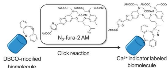
**Fig. 1** Chemical structure of N<sub>3</sub>-fura-2 AM and schematic illustration of the copper-free click reaction with dibenzylcyclooctyl (DBCO)-modified biomolecules.
