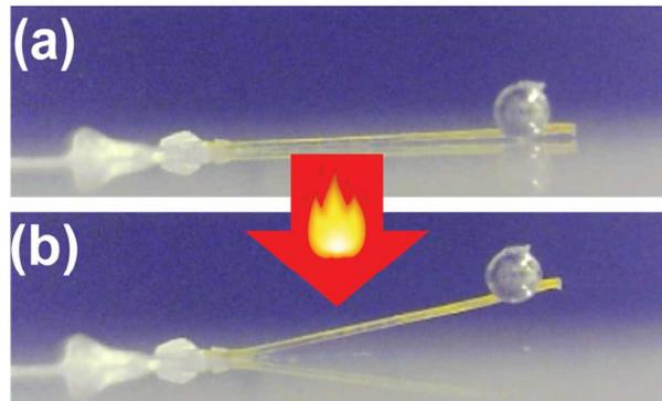
cantilever is about 0.01  $\mu\text{J}$ , and the force generated from the  $\alpha$ -phase to the  $\beta$ -phase transition is 40  $\mu\text{N}$ .
