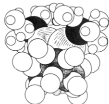
Figure 5. Space-filling diagram of isomer II of \text{HFe}_4(\text{CO})_{12}\text{Au}_3\text{PET}_{3/2}\text{B} , viewed along the iron butterfly wing-wing axis. The ethyl groups are oriented as determined from the X-ray diffraction data.
